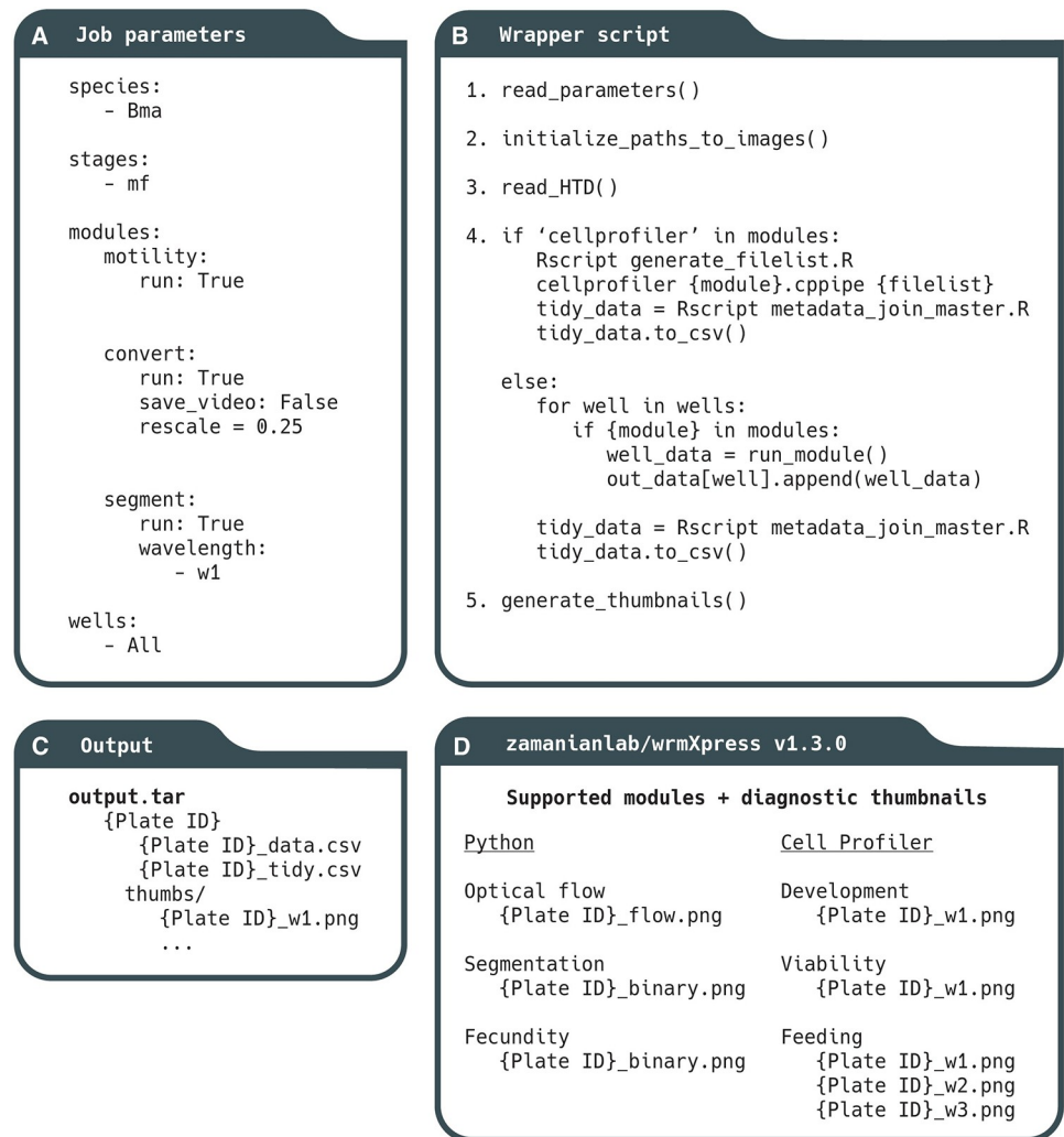
Fig 2. Constituents of the wrmXpress workflow. (A) Jobs are parameterized with a user-generated YAML file, which includes species and stage information, and allows for the selection of Python or CellProfiler modules. (B) The wrapper script controls the implementation of wrmXpress. (C) Output data includes raw data, raw data with joined metadata, and diagnostic thumbnail images. (D) wrmXpress comes packaged with 6 distinct analytical modules.
